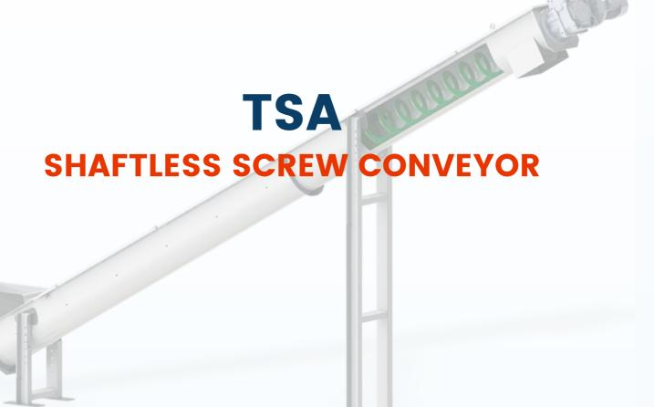
Built by a shaft less screw that rotates to the inside of a trough (tubular or U-section) with one or more loading hoppers and one or more exhaust mouths. The rest of the machine is closed by covers. The absence of the inner shaft allows the transport of sticky materials, usually difficult to transport by the screw with shaft. The bottom of the trough is being protected by a wearresistant coating in HDPE or steel depending on the material to be conveyed.
